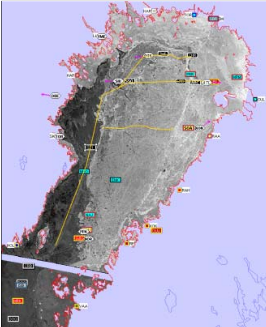
Figure 3. An example of the IBPlott image showing the Bothnian Bay, suggested ship routes and location of icebreakers and merchant vessels (source: VTT Information Technology Web page).
